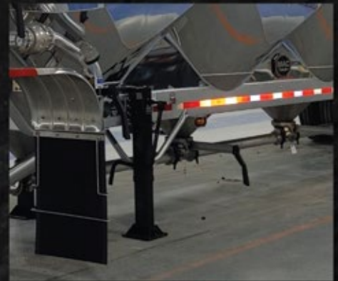
Industry leading 15" piping ground clearance with lowest possible overall vehicle height.
