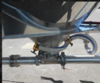
Food Grade Aerators and Hoses
