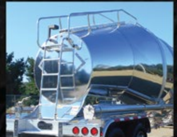
Transition Walkway with Handrails
