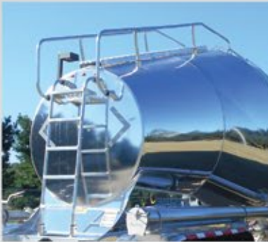
Transition Walkway with Handrails
